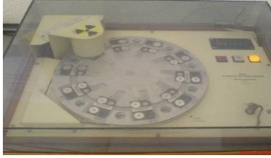
Fig. 3: Type 623 Dosimeter Irradiator with Sr/Yr-90 source
