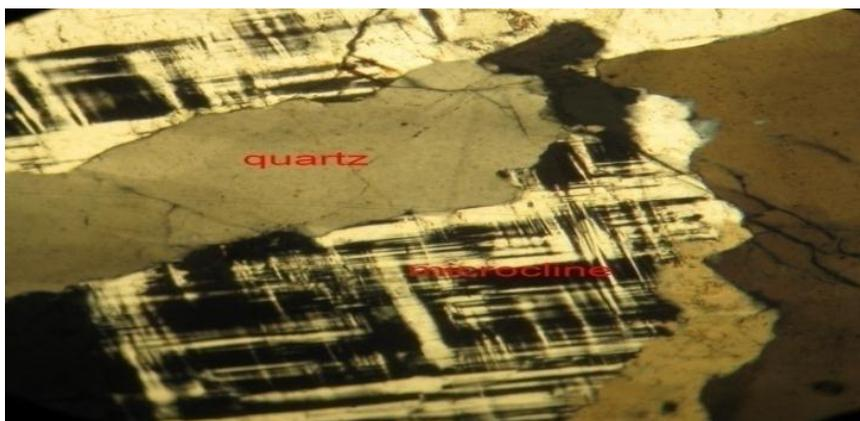
Fig. 5. Photomicrograph of porphyritic granite from Isan Ekiti using 40X magnification
