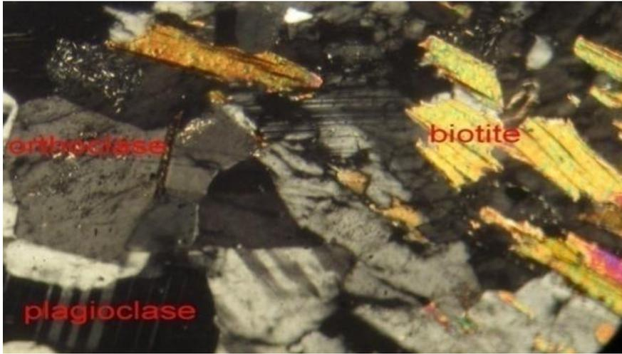
Fig. 6. Photomicrograph of fine to medium-grained granite from Isan Ekiti cpl 40X
