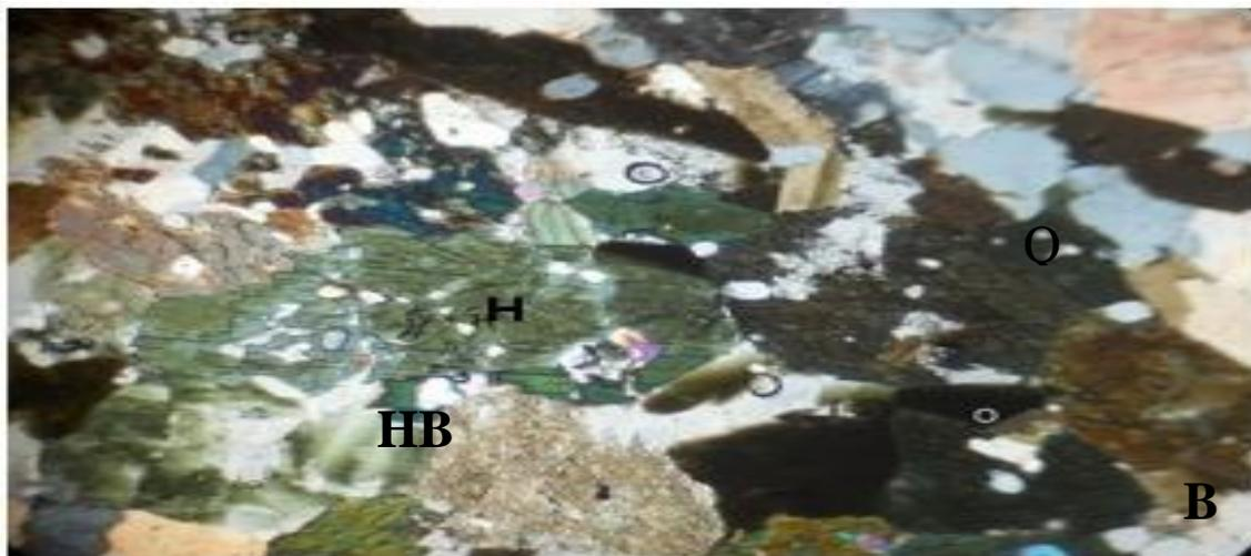
Fig. 4: Photomicrograph of charnockite from Isan Ekiti. 40X magnification showing H=Hypersthene, HB=Hornblende, B=Biotite and Q=Quartz
